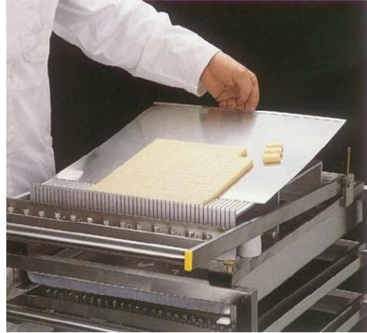
The pralines cutter have been specially studied for professionals whose want a reliable a simple material to use. It allows cutting the recipe easier and quickly. Change a frame is very fast with the new system to block it and the color different by frames.
